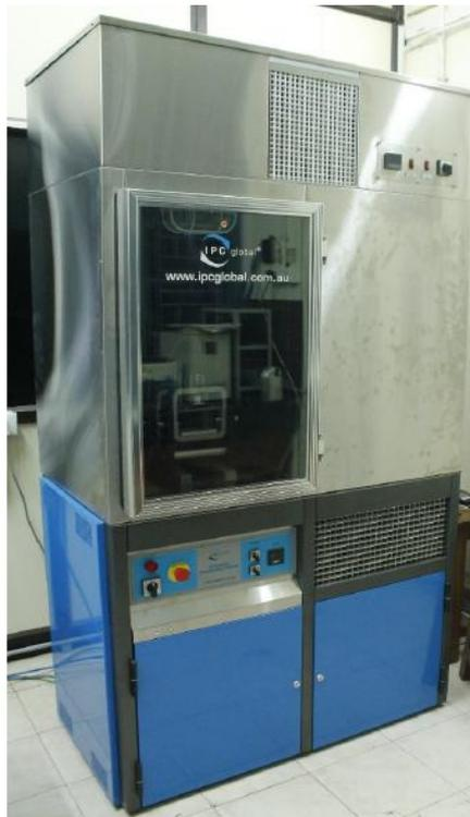
Figure 3.14: Four point beam bending equipment
